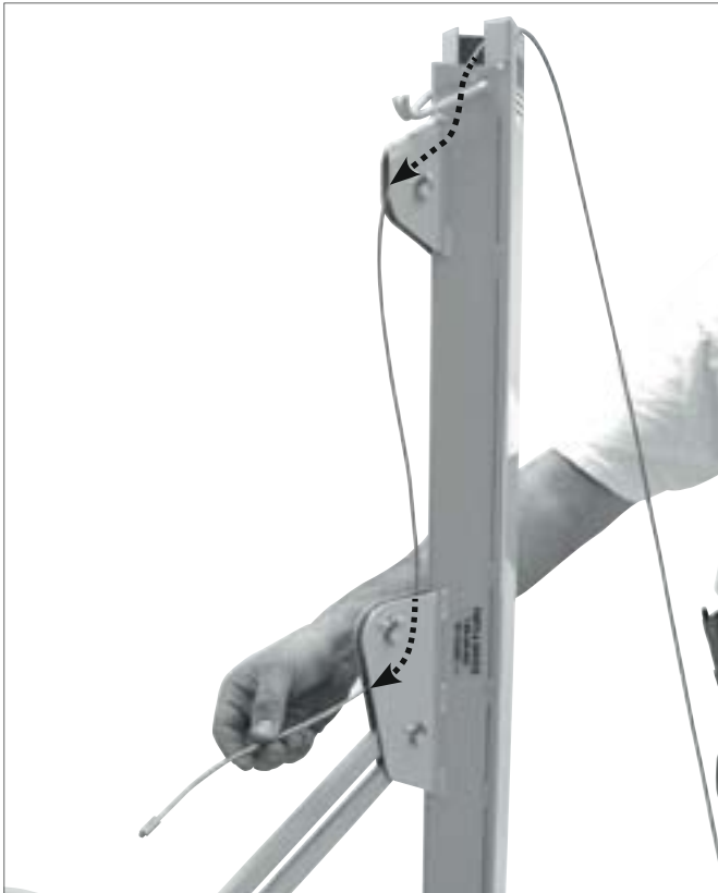
27. A correctly threaded cable for the Panellift® Model 182 is shown above.
