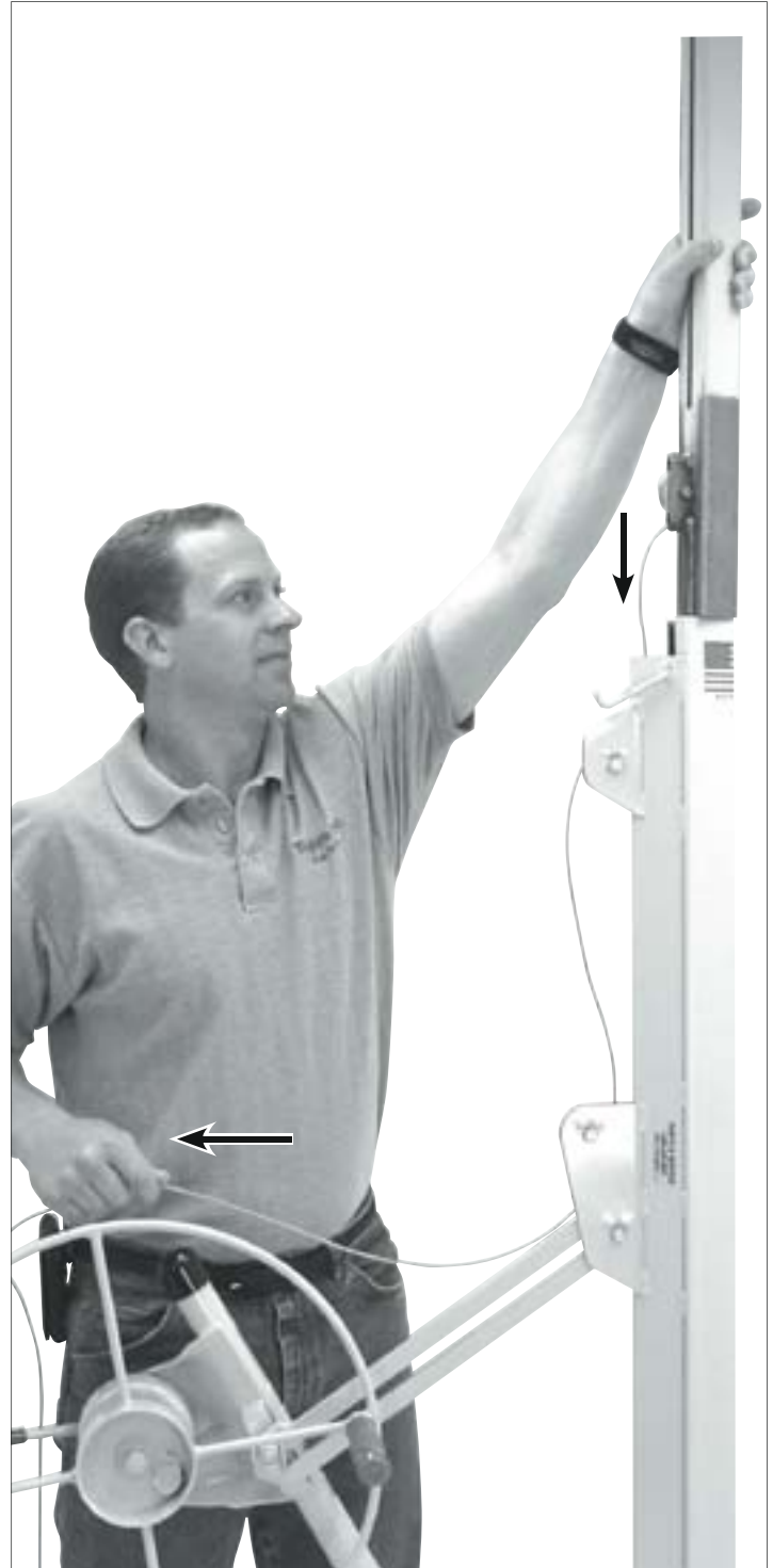
28. Pull the slack cable through the sheave pocket toward the winch and slide the telescoping sections into the frame housing. As the telescoping sections lower into the frame housing, the slack cable will be drawn back through the sheave pocket.
