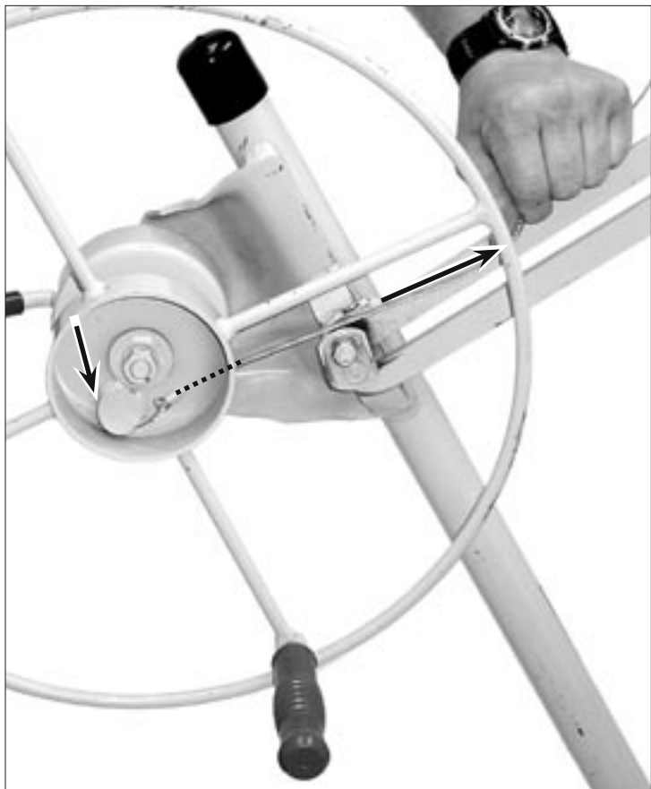
29. Feed the copper crimped end of the cable through the winch drum and secure it behind the mooring tab by hand pulling the cable snug as shown.
